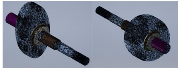
Figure 13: Mesh of finite elements in the model.
